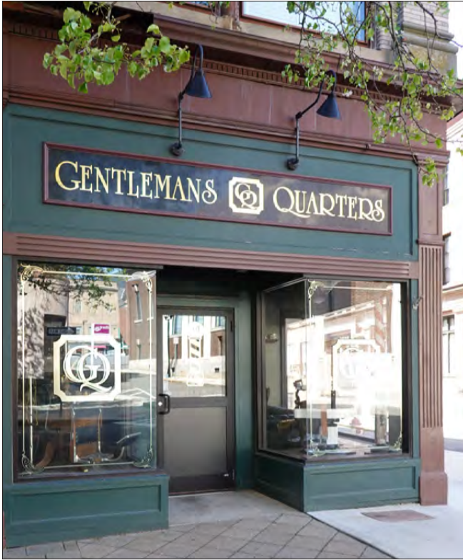
The clear lettering and strong contrast between the letter color and background make this sign very legible. Discrete gooseneck lights located above the sign provide illumination of the sign in the evening.
